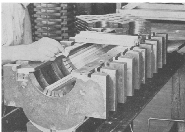
Fig. 16. V. D. Anderson Company horizontal barrel showing lining of barrel with barrel bars.
